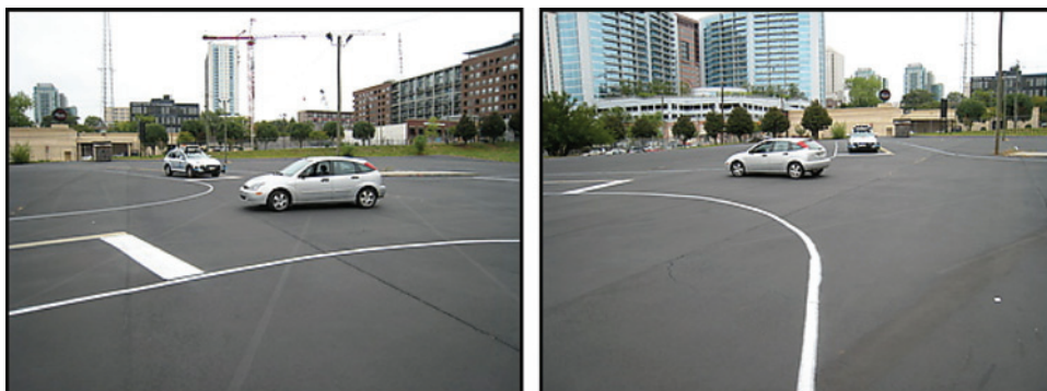
Fig. 10 An intersection is traversed by first establishing the correct precedence and then waiting for precedence, as part of the traverse intersection mode of operation.
